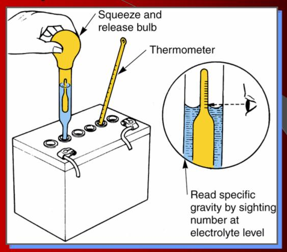
Electrolyte is sulfuric acid. Do Not Drip on clothes, skin or a vehicles finish. Flush with cool water if any splashes in your eyes!
