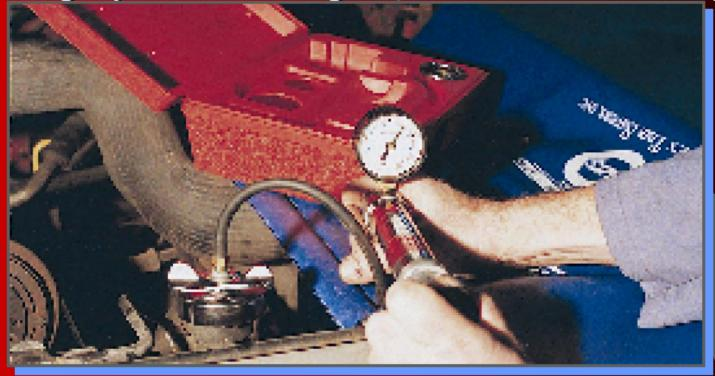
Performing a cooling system pressure Test. Never exceed radiator pressure cap pressure!
