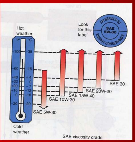
SAE oil viscosity rating is affected by temperature. Note how thicker oil (higher SAE number) is specified for higher outside temperatures
