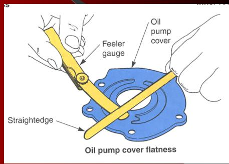
Measuring Oil Pump Cover and Gear (Rotor) Thickness
