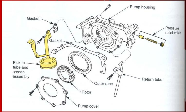
Exploded view of an oil pump that is mounted to the front of an engine.
