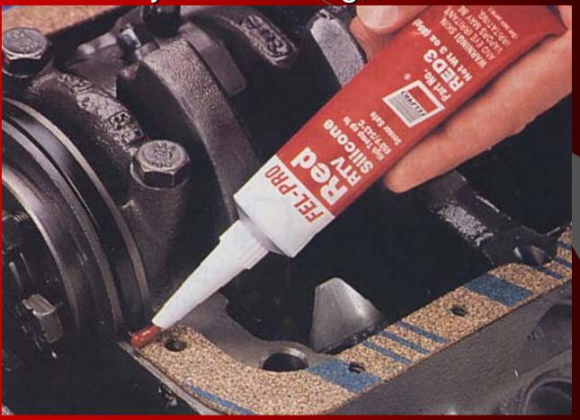
Installing RTV where the gasket meets a rubber seal. This is to prevent leakage
