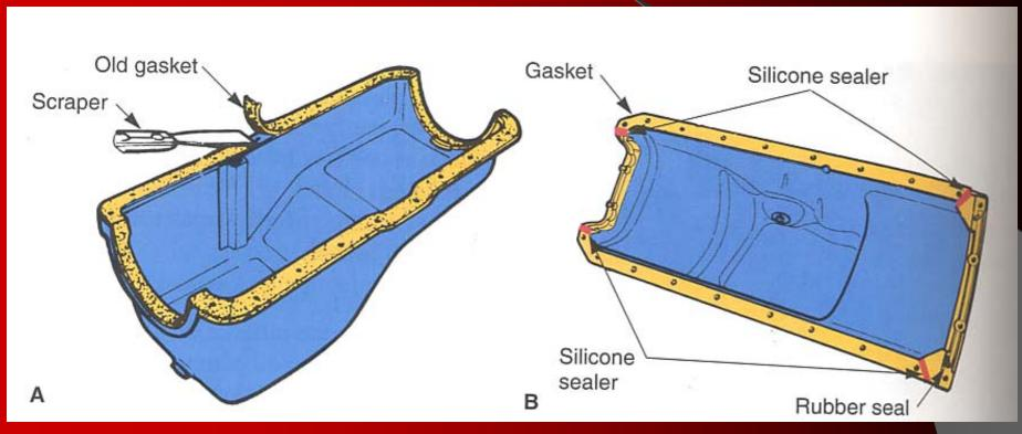
Using a gasket scrapper to remove an old, stuck old stuck-on gasket
