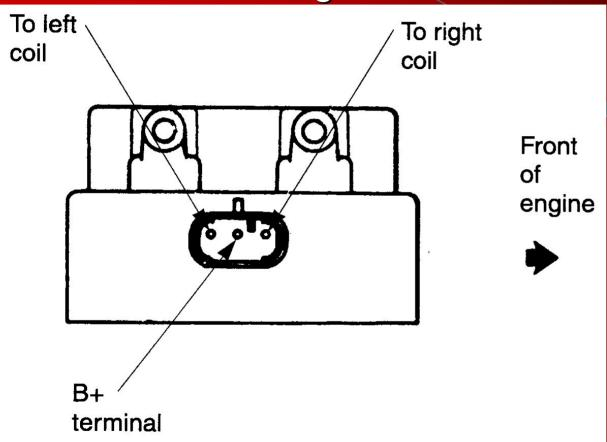
To check primary resistance, connect ohmmeter between B+ terminal and the pin corresponding to the coil in question.
