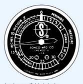
Intake manifold air leak
