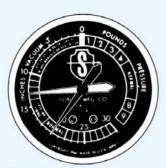
Burned or leaky valves Burned valve will cause pointer to drop every time burned valve opens.
