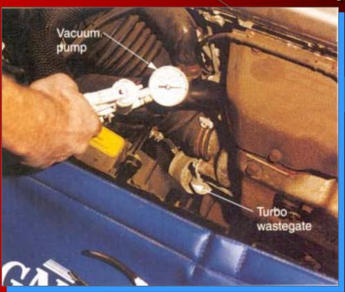
Used to check vacuum-actuated devices and vacuum diaphragms
