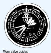
If pointer fluctuates excessively at idle but steadies at higher speeds, valves may be worn allowing air to upset fuel mixture.
