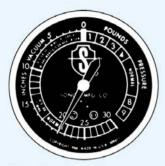
Normal engine reading Vacuum gauge should have reading of 18-22 inches of vacuum. The needle should remain steady.
