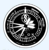
Weak valve springs Vacuum will be normal at idle but pointer will fluctuate excessively at higher speeds.
