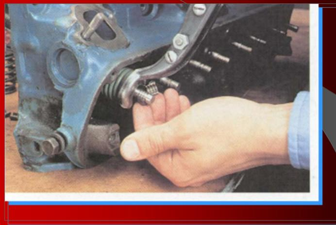
With the valve springs compressed, keepers can be removed
