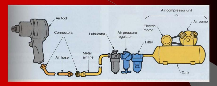
The basic parts of a typical automotive repair shop air pressure system
