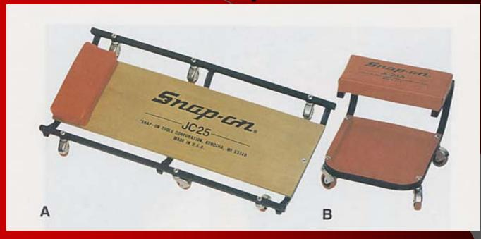
Creepers are very useful when working under a vehicle. NEVER leave a creeper lying on the floor: a person can easily trip or fall over it and get injured.
