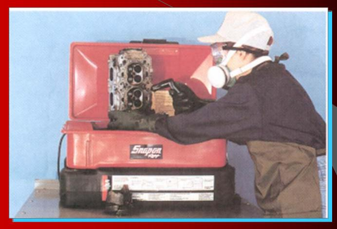
Contains a pump, reservoir, and solvent—used to remove grease and oil from parts
