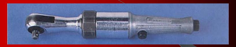
An Air Ratchet is a special impact tool designed to work in areas with limited space or access. Always "break" the fastener by hand before using the air ratchet to remove the fastener. ALWAYS wear safety glasses when using any air powered impact tool!
