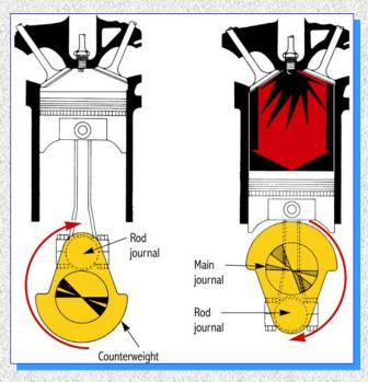
Counterweight offsets the weight of the piston and rod to prevent vibration
