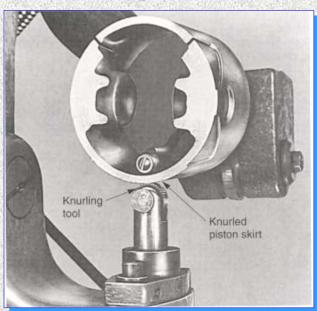
Increases skirt diameter by squeezing metal outward around small dents
