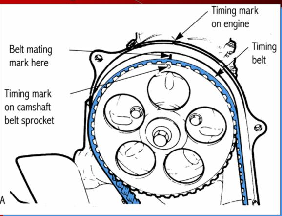
The camshaft sprocket mark is aligned with the belt marking and the timing mark on the engine
