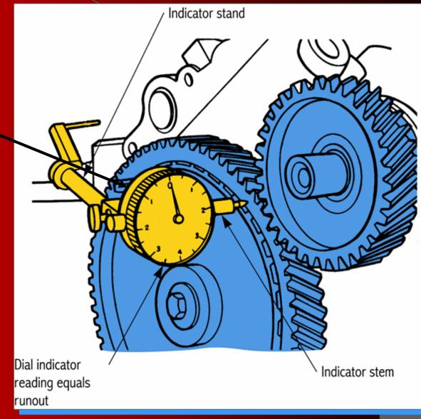
Measuring timing ear runout using a dial indicator
