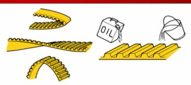
A-Do not bend, twist, or turn belt excessively. Oil and water will deteriorate belt. Fix all engine leaks.
