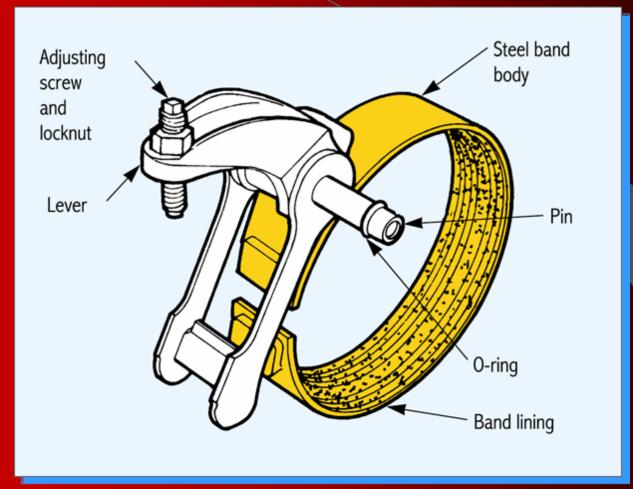
One end is anchored to the case
