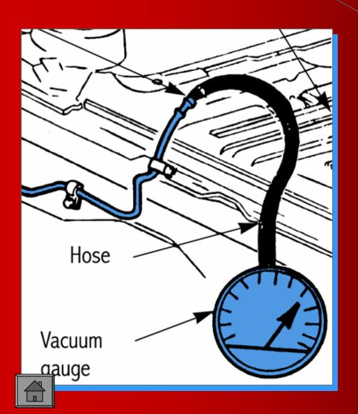
Connect a vacuum gauge to the modulator line with a T-fitting; with engine idling, reading should match manifold vacuum (high and steady)
