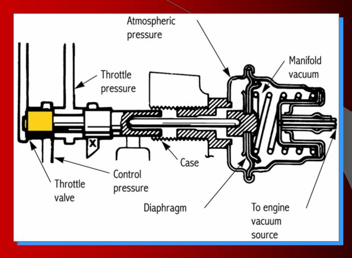
Under high load, valve delays up shifts
