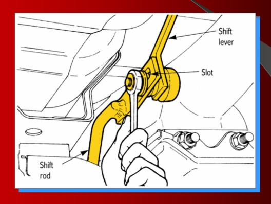
Position the shifter and the lever on the transmission in the same gear
