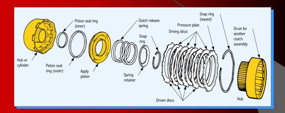
Driving discs are splined to hub. Driven discs are locked in the drum
