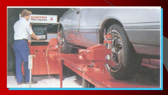
Specialized stall used when working on steering and suspension systems
