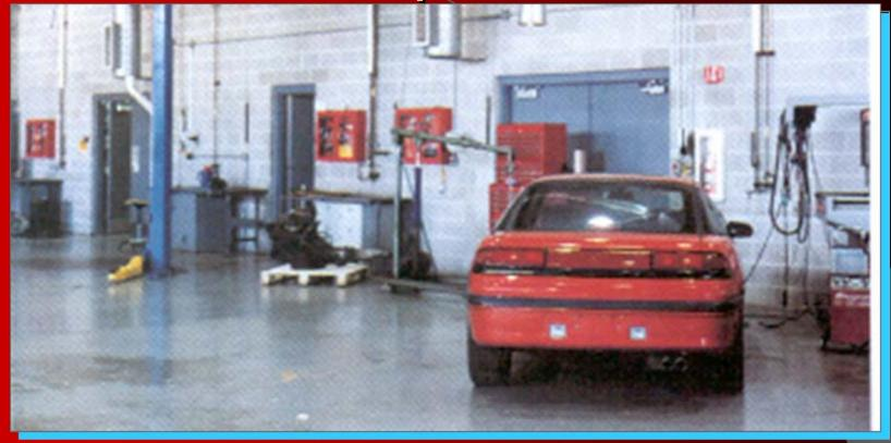
Work area where a car can be parked for repairs Sometimes stalls are numbered and marked off with safety lines painted on the floor
