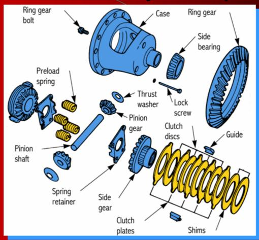
Amount of torque needed to make one axle or differential side gear rotate the limited-slip differential clutches
