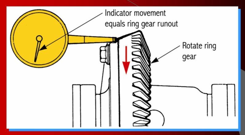
If runout is excessive, check ring gear mounting and case runout
