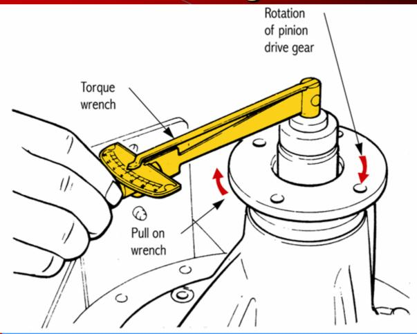
Measure preload with a torque wrench. Compare the measurement to specs
