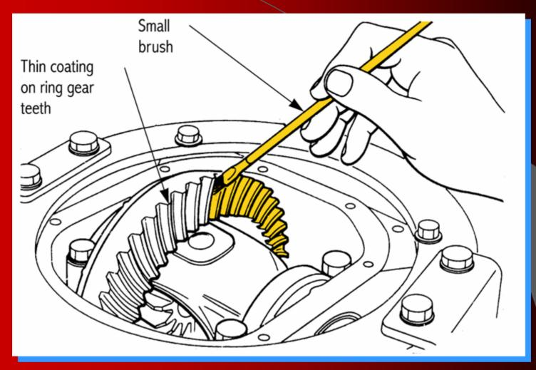
Checking gear contact pattern
