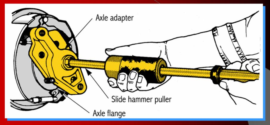
Using a slide hammer puller
