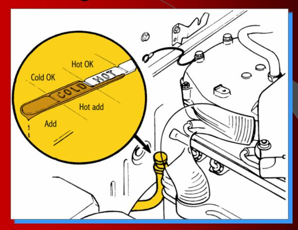
Fluid level should be between the add and full marks
