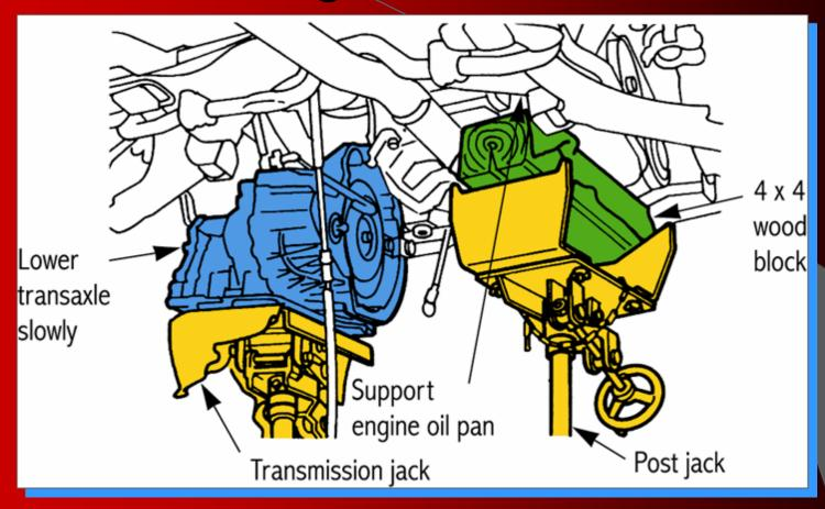
Using a transmission jack to remove the transaxle and a post jack to support the engine
