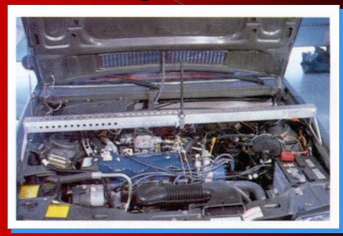
Engine holding fixture may be required to support the weight of the engine
