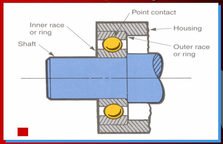
Balls allow parts to rotate with a minimum amount of friction and wear
