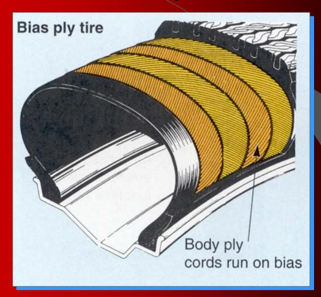
3. The tire TREAD is the outer surface of tire that contacts road.
