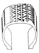
**D-One-side wear.** Here's another type of alignment problem-excessive camber, which means tire is leaning too much to inside or outside of tread, and placing all work on one side of tire.
