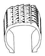
**A-Feathering.** This is caused by erratic scrubbing against road when tire is in need of toe-in or toe-out alignment correction.
