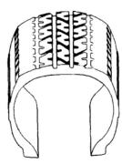
C-Underinflation. When a tire is underinflated, most of its contact with road is on outer tread rib, or shoulder, causing faster wear here than in middle. Be sure to check tire's air pressure.
