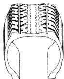
B-Overinflation. Overinflation can cause fast centerline wear in bias and bias belted tires. In this case, center ribs get more contact with road than they should and wear much faster than outer ribs.
