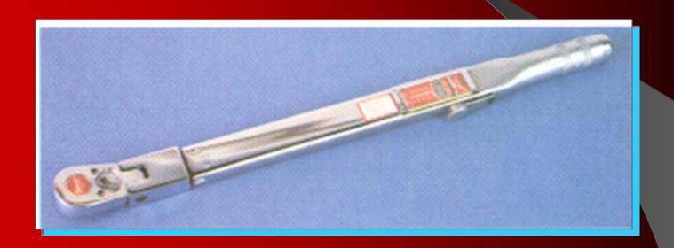
Torque value is set by turning the handle—fastener is tightened until it clicks
