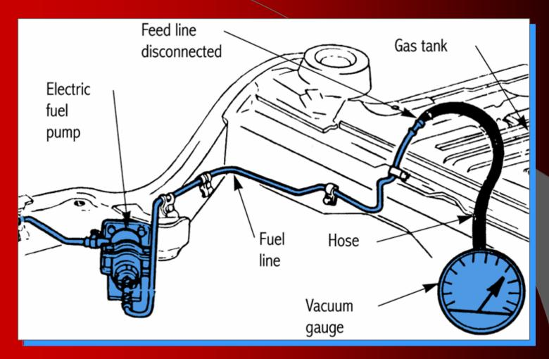
Connect a vacuum gauge to the inlet - the negative pressure side of the pump
