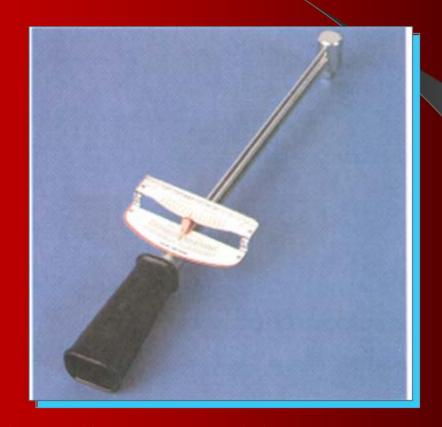
Uses a bending metal beam to make the pointer read torque on the scale
