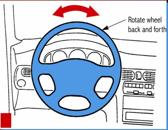
With the vehicle on the ground, rotate the steering wheel back and forth while someone watches for part wear
