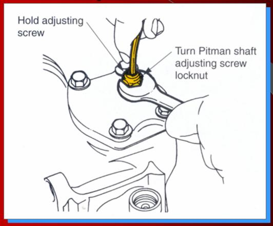
Loosen the locknut and bottom the adjustment screw lightly
