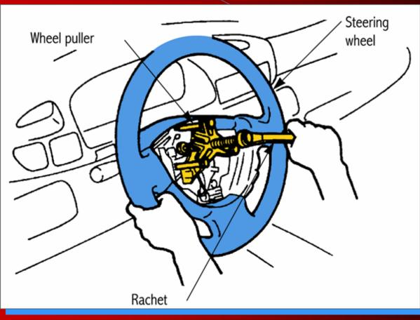
Tighten the puller down against the steering shaft to remove the wheel
