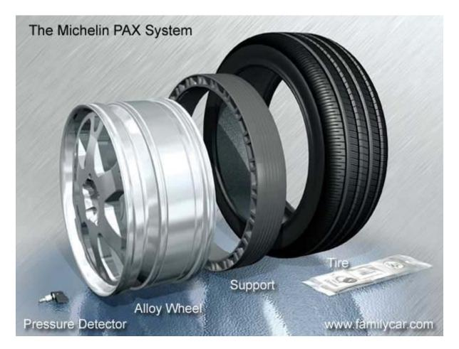
The PAX System includes a special wheel and tire that are designed to work together. There is also a support ring that fits around the center of the rim and supports the tire when it is deflated so that the vehicle can be driven. Another part of the system is the combination air valve / pressure detector which reports pressure loss to an indicator on the dash so that the driver knows that there is a problem.
