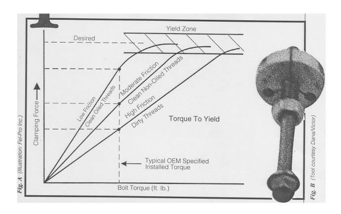
**Fig A.** Although the torque-to-yield procedure provide a more uniform clamping force, it permanently stretches the bolt. Reusing stretched bolts can lead to sealing (gasket) problems, which is why using recommended TTY bolts is highly-recommended.
