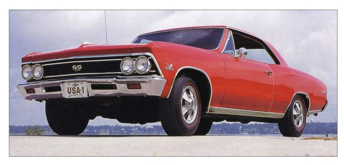
Like other GM intermediates, it was reskinned, though dimensions hardly changed. SS models got a blackout grille and a new hood with nonfunctional vents. With engines of around 400 cid now obligatory in this game, Chevy made the 396-cid V-8 standard, so all its midsize muscle cars were now Chevelle SS 396s.
