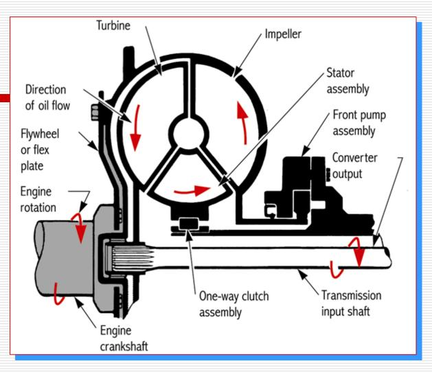
Connects torque converter to the driving components in the transmission
