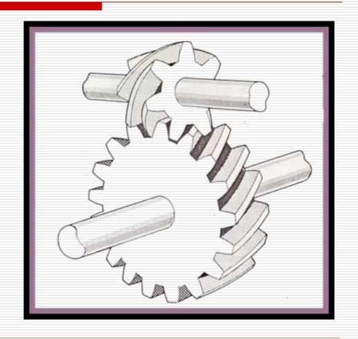
Straightcut gear teeth are NOT quieter than helical gears and DO cause axial thrust.
