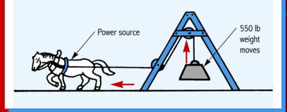
One horsepower equals 33,000 ft lb of work per minute
