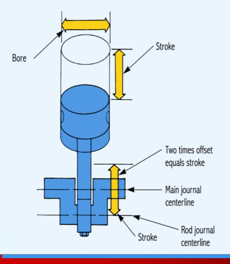
Bore • Diameter of the engine cylinder Measured across the cylinder, parallel with the top of the block
