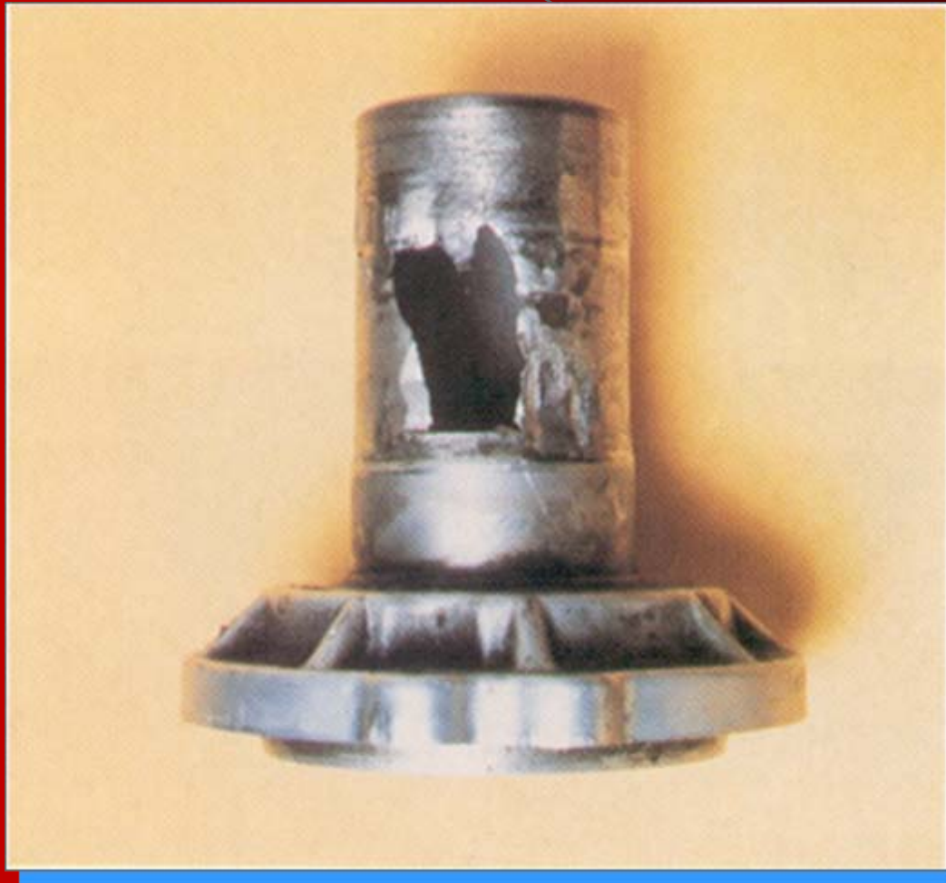
Damaged Bearing Retainer Hub
