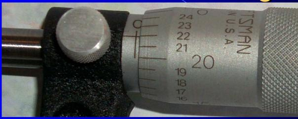
What is the **largest number** visible on the **micrometer barrel**? How many **graduation lines** to the right of the sleeve number? What is the **thimble graduation** aligned with the horizontal sleeve line? Add the three readings...
