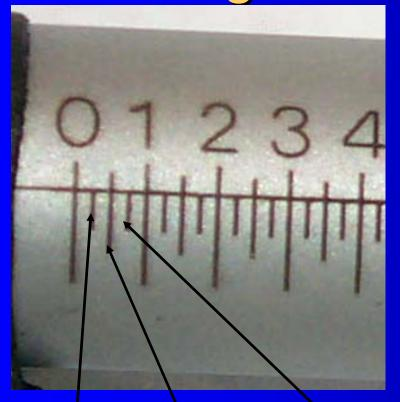
Count the number of graduation lines to the *right* of the barrel number. Each full sleeve graduation equals 0.025 (2 full lines = 0.050, 3 = 0.075)
