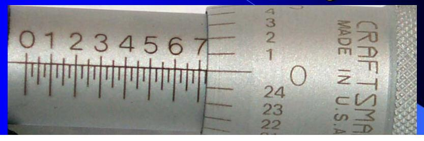
What is the **largest number** visible on the **micrometer barrel**? How many **graduation lines** to the right of the sleeve number? What is the **thimble graduation** aligned with the horizontal sleeve line? Add the three readings...
