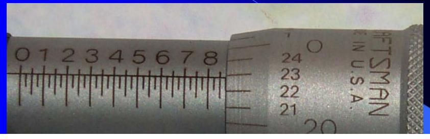
What is the **largest number** visible on the **micrometer barrel**? How many **graduation lines** to the right of the sleeve number? What is the **thimble graduation** aligned with the horizontal sleeve line? Add the three readings...
