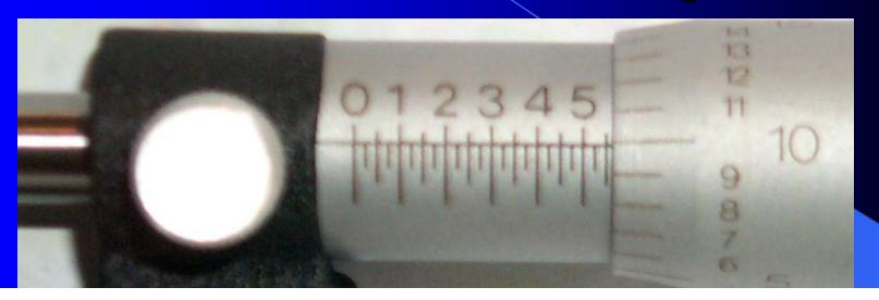
What is the **largest number** visible on the **micrometer barrel**? How many **graduation lines** to the right of the sleeve number? What is the **thimble graduation** aligned with the horizontal sleeve line? Add the three readings...
